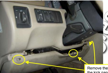
The module is located above the kick panel. It's attached to steering column under the dash.
